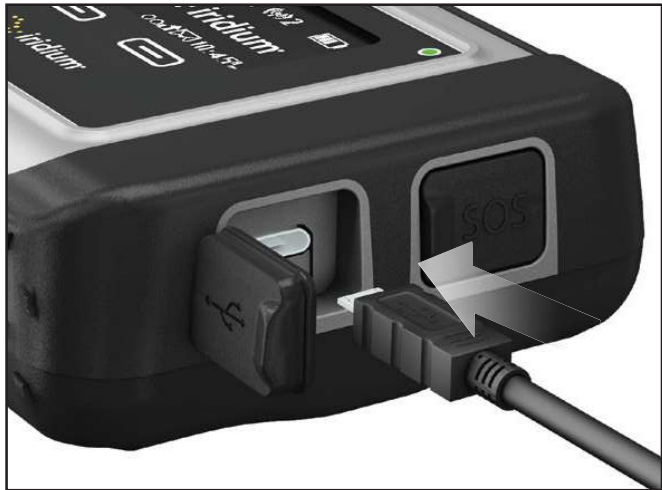
Charging the battery
